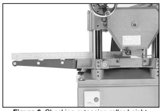
Figure 6. Checking extension roller height.
